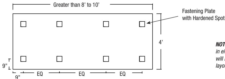
**NOTE:** Less than 3'-6" in either direction will require a custom layout.
