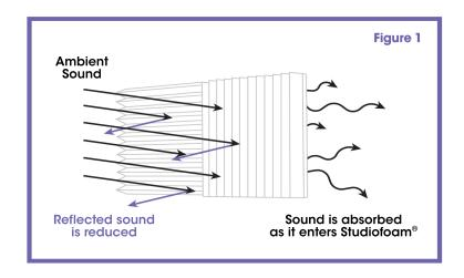
How well a product absorbs sound is based on many conditions, such as the type of material, it's thickness and shape. The properties of absorption also change based on frequency. High frequencies are more easily absorbed than low frequencies. These are measured at 1/3<sup>rd</sup> octaves and their performance is called its absorption coefficient.
