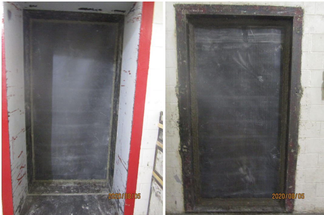
Figure 1 – Specimen mounted in test opening, as viewed from source room (left) and receive room (right)
