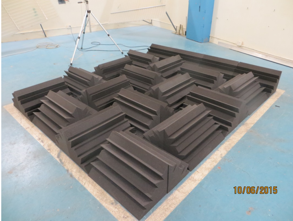
Figure 1 - Specimen mounted in the test chamber.
