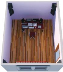
The first step for acoustic treatment in any small room should be to place Bass Traps in all of the corners.
