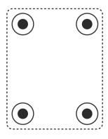
To maximize the performance, of your ProPODs, place each decoupler 1" inside each corner of your monitor, loudspeaker, subwoofer, turntable or other audio component weighing up to 50lbs. (22.68kg)
